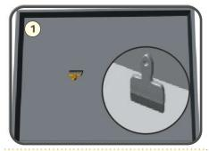
Clean up debris on the mounting surface to ensure surface cleaning
