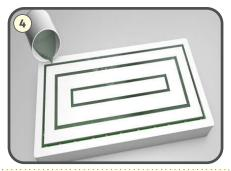
After the module is initially installed, it is sealed with epoxy glue.
