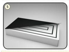
After the epoxy glue is dried, then backlight shading treatment is performed with a reflector.
