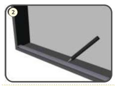
Determine the installing position for modules and the needed qty. Make sure to install it close to the bottom of the light box.
