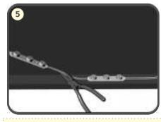
Cut off the modules to the desired qty, and peel off the insulation skin of wires about 10 mm
