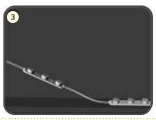
Peel off the release paper of double-sided adhesive tapes, then, stick modules on the installing surface for preliminary mounting.
