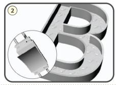
Peel off the release paper of double-sided adhesive tapes, then, stick modules on the installing surface for preliminary mounting
