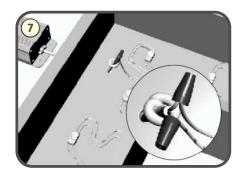
Please ensure that the '+' and '-' of the wires of modules are connected with those of power supply correctly, and dispose with waterproof, insulation, anti-circuit and anti-corrosion protection.
