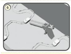
Adjust the modules to the best position, press the double-sided tape tightly and then fix by neutral glass glue
